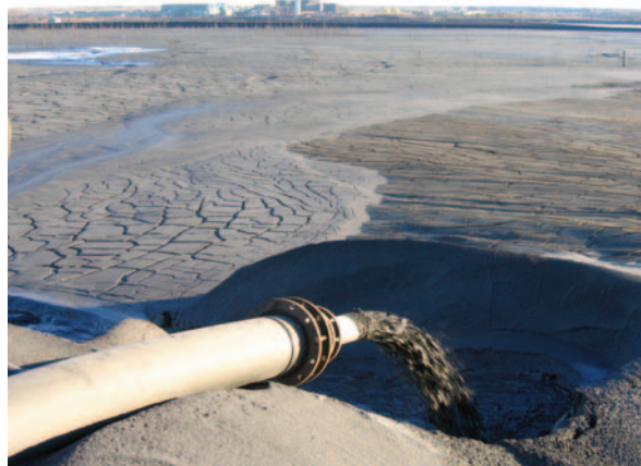
FIGURE 3 Mine tailings disposal at Kidd Creek, Ontario, Canada. The Kidd metallurgical facility, which ceased operations in 2010, is shown in the background. PHOTO BY BERND LOTTERMOSER
